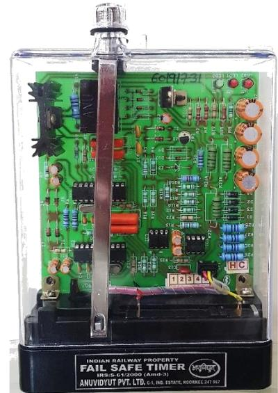
Working of the device is indicated through red blinking LEDs on the control card which are easily visible from outside and a green LED is provided to indicate completion of time delay cycle.
